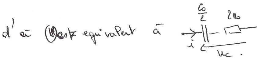
b) Généralisation:  $C_{eq} = \frac{C_0}{m}$   $R_{eq} = m R_0$ .
