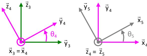
$$\vec{V}_{P \in 6/3} = \frac{d}{dt} \vec{O_3 P} \Big|_3 = \frac{d}{dt} \vec{O_3 O_4} + \vec{O_4 O_5} + \vec{O_4 P} \Big|_3 = \frac{d}{dt} a_4 \cdot \vec{x}_3 + a_5 \cdot \vec{x}_5 + a_6 \cdot \vec{x}_5 \Big|_3 = (a_5 + a_6) \cdot \frac{d}{dt} \vec{x}_5 \Big|_3$$
