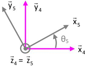
$$\vec{V}_{P \in 6/4} = \frac{d}{dt} \vec{O_4 P} \Big|_4 = \frac{d}{dt} \vec{O_4 O_5} + \vec{O_4 P} \Big|_4 = \frac{d}{dt} a_5 \cdot \vec{x}_5 + a_6 \cdot \vec{x}_5 \Big|_4 = (a_5 + a_6) \cdot \dot{\theta}_5 \cdot \vec{y}_5 \rightarrow \boxed{\vec{V}_{P \in 6/4} = (a_5 + a_6) \cdot \dot{\theta}_5 \cdot \vec{y}_5}$$
