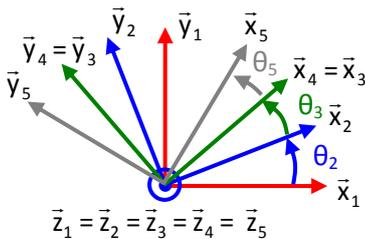
$$\vec{V}_{P \in 6/1} = \frac{d}{dt} \vec{O_1 P} \Big|_1 = \frac{d}{dt} \vec{O_1 O_2} + \vec{O_2 O_3} + \vec{O_3 O_4} + \vec{O_4 O_5} + \vec{O_4 P} \Big|_1 = \frac{d}{dt} a_2 \cdot \vec{x}_2 + a_3 \cdot \vec{x}_3 + a_4 \cdot \vec{x}_3 + a_5 \cdot \vec{x}_5 + a_6 \cdot \vec{x}_5 \Big|_1$$
