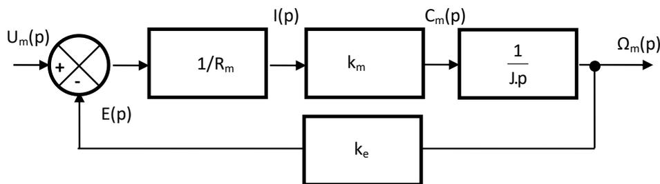
**Q.3.**  $\frac{\Omega_m(p)}{U_m(p)} = \frac{1}{k_e} \cdot \frac{\frac{k_m.k_e}{R_m.J.p}}{1 + \frac{k_m.k_e}{R_m.J.p}} = \frac{1}{k_e} \cdot \frac{k_m.k_e}{R_m.J.p + k_m.k_e} = \frac{1}{k_e} \cdot \frac{1}{1 + \frac{R_m.J}{k_m.k_e} p} = \frac{K}{1+T.p}$  avec  $K = \frac{1}{k_e}$  et  $T = \frac{R_m.J}{k_m.k_e}$
