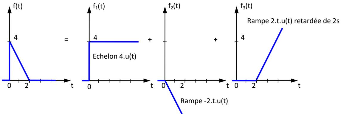
$$f(t) = f_1(t) + f_2(t) + f_3(t) \rightarrow F(p) = F_1(p) + F_2(p) + F_3(p) = \frac{4}{p} - \frac{2}{p^2} + \frac{2}{p^2} \cdot e^{-2p}$$
