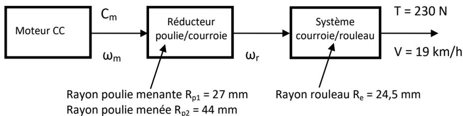
On a  $\frac{\omega_r}{\omega_m} = \frac{R_{p1}}{R_{p2}}$  et  $V = R_e \cdot \omega_r \rightarrow \omega_m = \frac{R_{p2}}{R_{p1}} \cdot \omega_r = \frac{R_{p2}}{R_{p1}} \cdot \frac{V}{R_e}$
